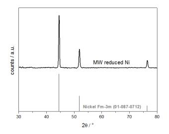
Figure 1. Powder X-ray diffraction of the MMN.
