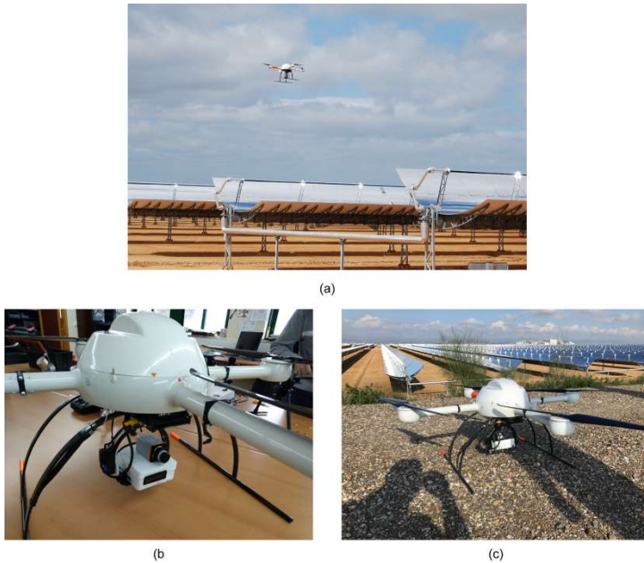
Figure 6. (a) The UAV performing an inspection on CSP plant, (b) front view of system onboard the UAV, (c) back view of system onboard.
