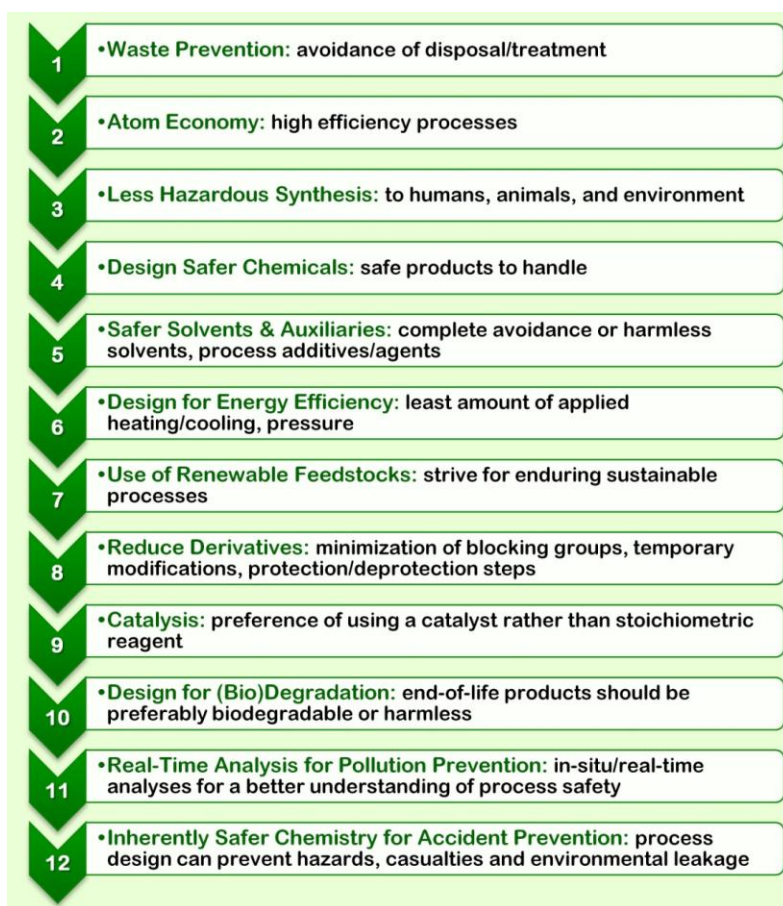
Figure 3. The 12 principles of Green Chemistry developed by P. T. Anastas and J. C. Warner. Adapted from reference. 21
