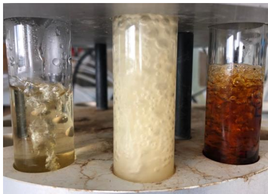
Figure 1. Reactions performed in solvent after 1.5 h (Left to right: blank, alumina catalyzed, Amberlyst-15 catalyzed)
