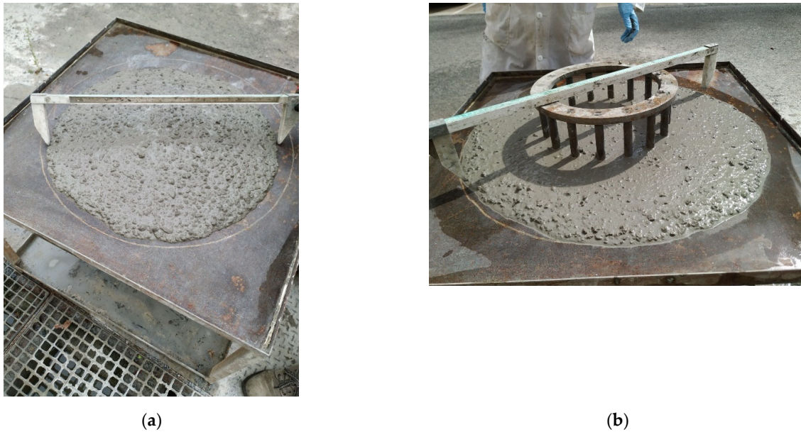
Figure 4. Results of the tests carried out according to the current regulations for considering self-compacting concrete (EHE-08). Slump flow (a) and J-Ring (b).
