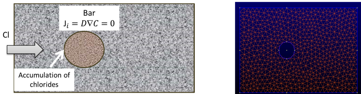
Figure 1. (Left) Rebar is acting as a barrier against the chloride diffusion where J_c is the chloride flux. (Right) Mesh used.
