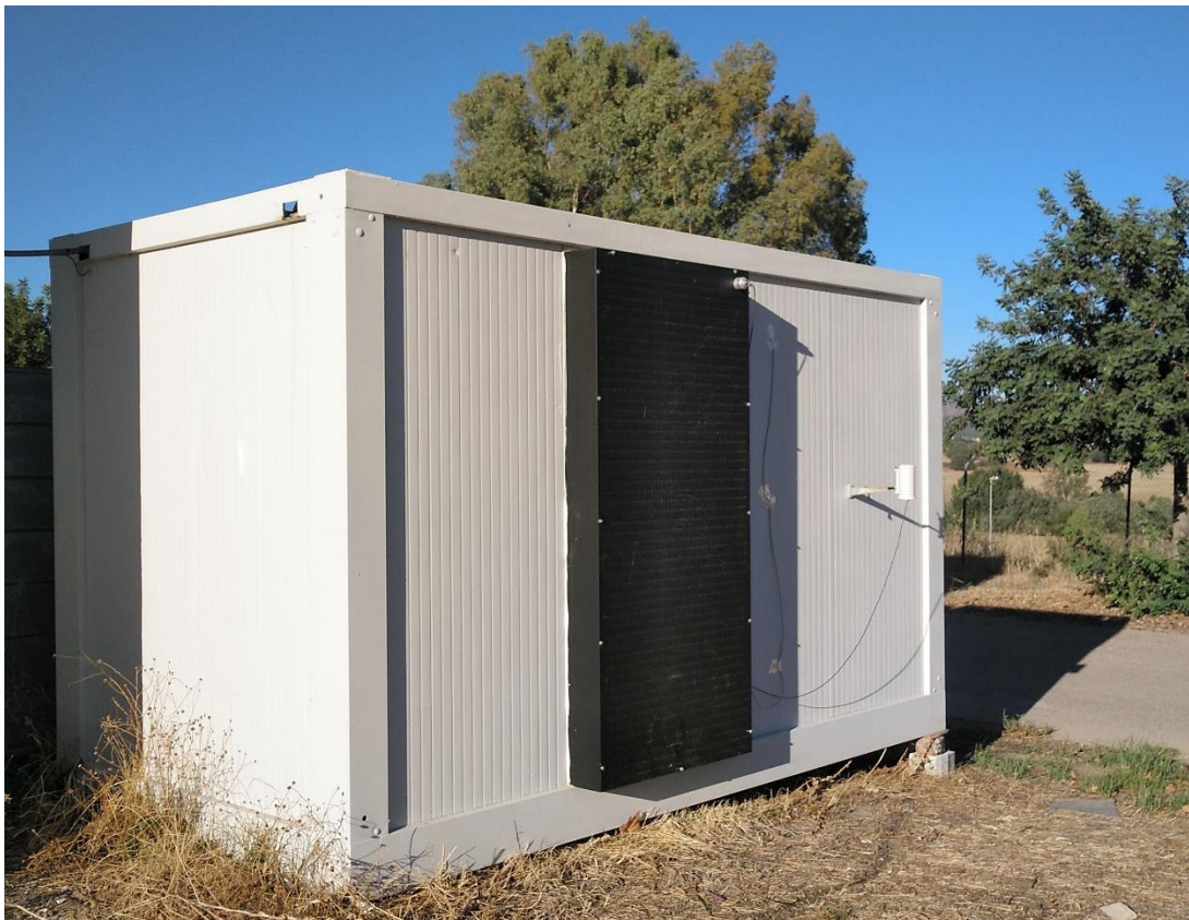
120 Figure 2. The test cell. The position of the UTC façade module, the surface temperature probes and the protected ambient 121 temperature probe (right) can be seen.
