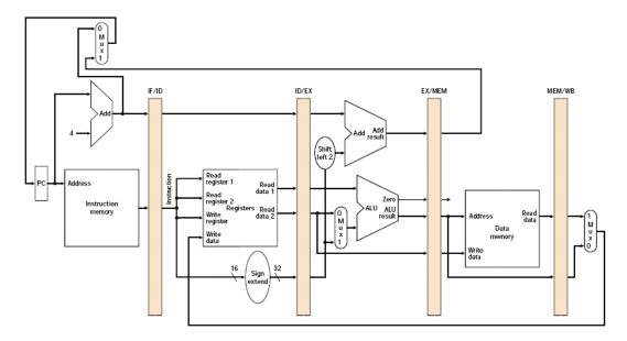
Figure 1. Pipelined version of the MIPS datapath.
