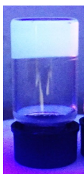
Figure S1. Image of c-NC hydrogel at 9 wt% undergoing the inversion test under UV light.
