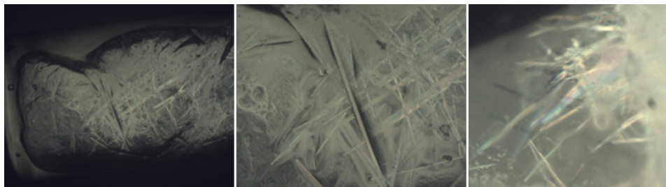
Figure S5. Crystals of the octadecylammonium salt of sulfamethoxazole 1:2 DMSO solvate obtained in OD/c-NC gels.
