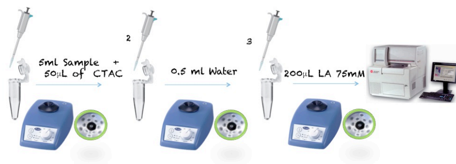
Figure VI.5. Scheme of the analytical procedure for the determination of AgNPs using s-NC as sorbent material.
