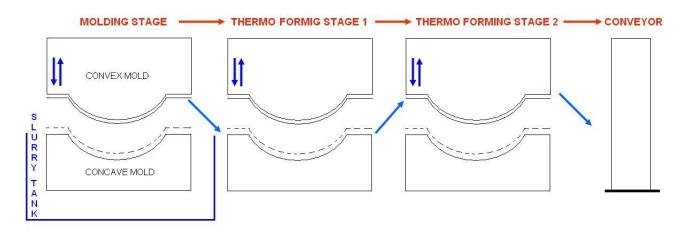
Fig. 3. The thermoformed process of containers manufactured from cellulosic pulps from cereal straw
