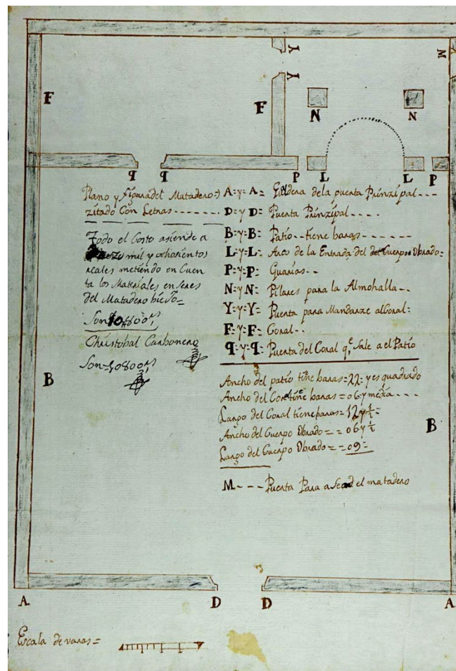
Figure 7. Plan of the slaughterhouse with the patio (B), animal pen (F), room (L), and building access [62].
