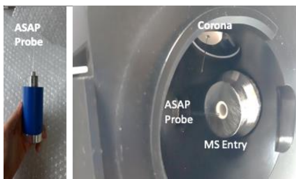
Figure S1. ASAP probe and APCI source used in this study
