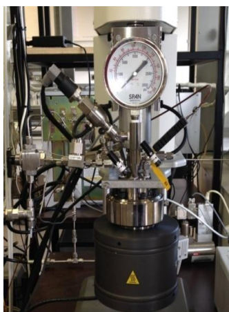
Figure 3. Reactor system used in APP of biomass derivatives solutions.
