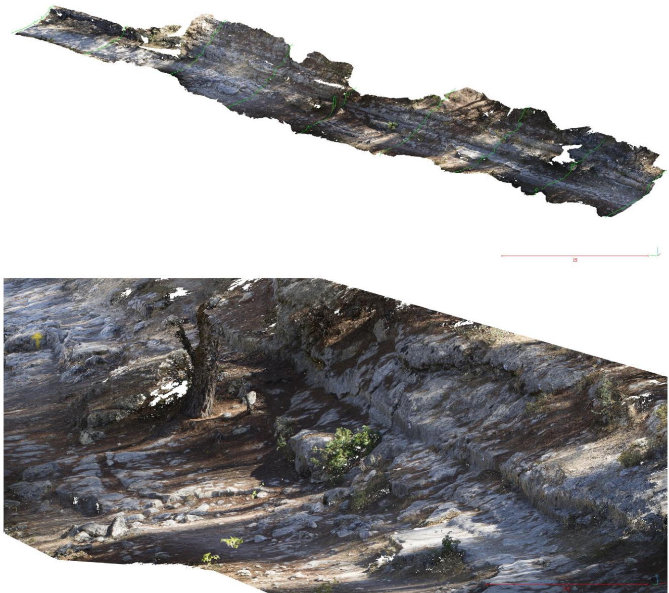
Fig. 8: a) Part of the dense point-cloud with polyline sections by photogrammetric survey of the Loma de los Escalones; b) detail of the roman road surface and the quarry by dense point-cloud (Massimo Gasparini for © Project Ager Mellariensis).
