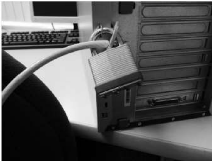
FIGURE 10.5 A cable can be used to keep a desktop machine from easily being taken.
