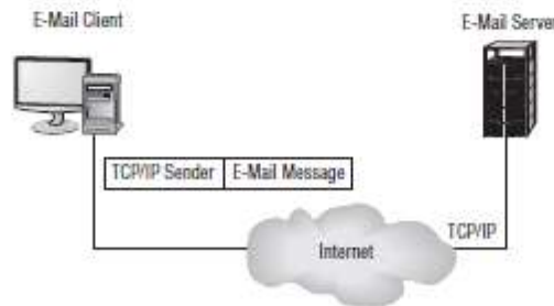
FIGURE 2.3 An email message that an email client sent to an email server across the Internet
