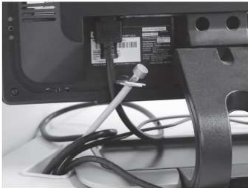
FIGURE 10.6 If theft of equipment is a possibility, run one end of the cable from the monitor to the desktop machine through the hole in the work desk.
