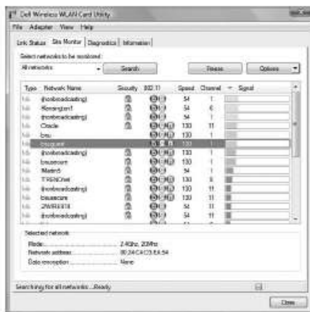
FIGURE 12.1 A number of wireless networks are found, and most are using more than one 802.11 standard
