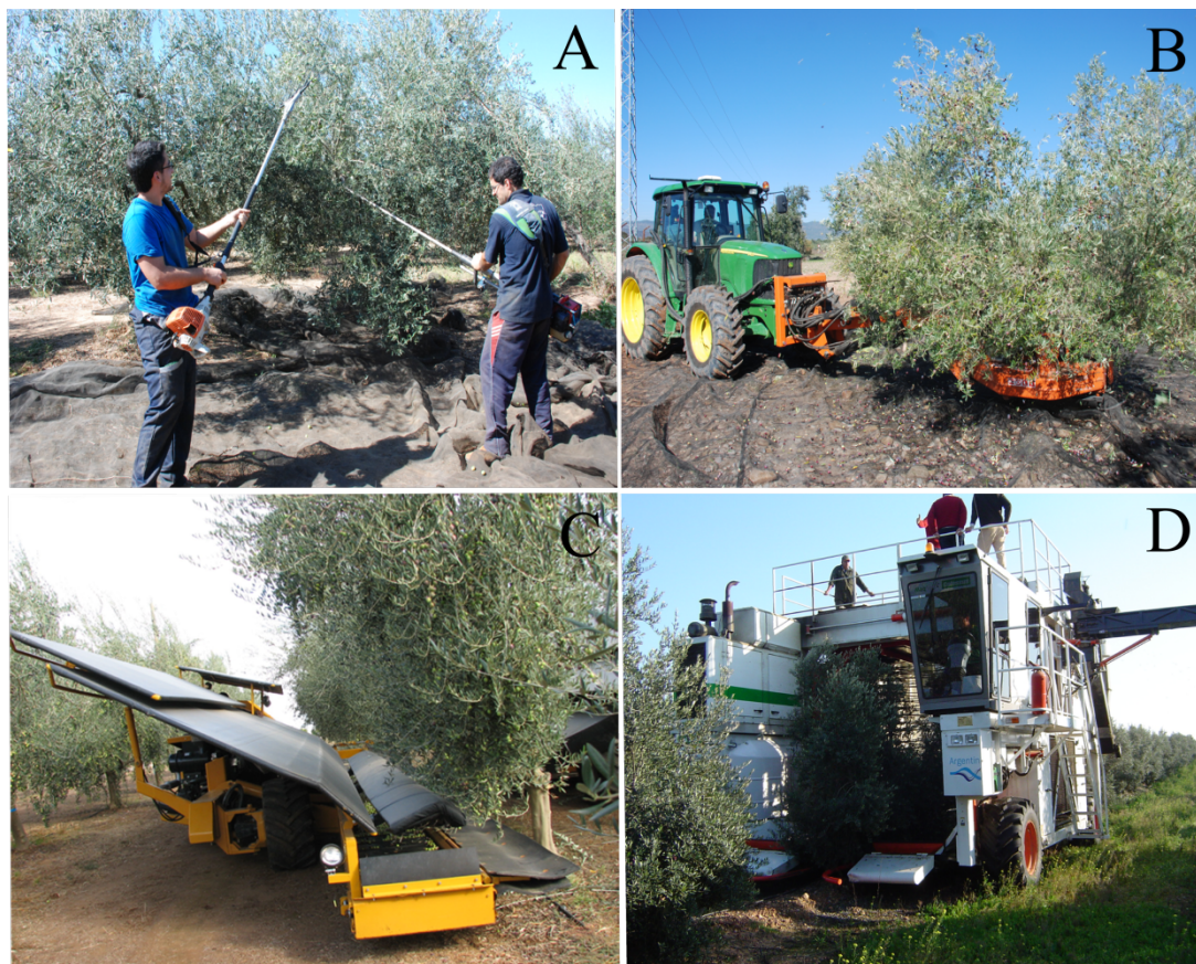
Fig. 24. Hand-held branch shakers removing fruit on nets (A); tractor-hitched trunk shaker on a high-density olive tree (B); side-by-side harvester detaching fruit using a trunk shaker and collecting them on a catch frame (C); and straddle harvester based on a canopy shaker collecting fruit on a catch frame (D)
