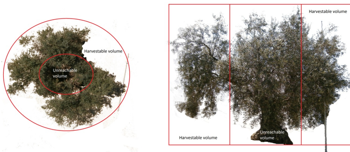
Fig. 32. Ring elliptical cylinder that determines the reachable canopy volume for canopy shakers.
