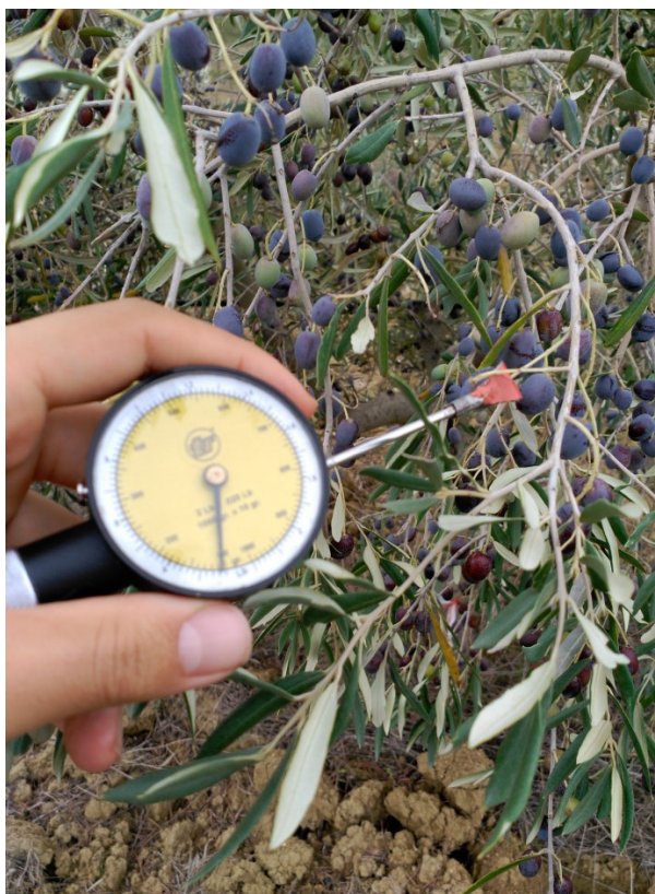
Fig. 37. Dynamometer with modified hook for apply stalk twisting before FDF measurement.
