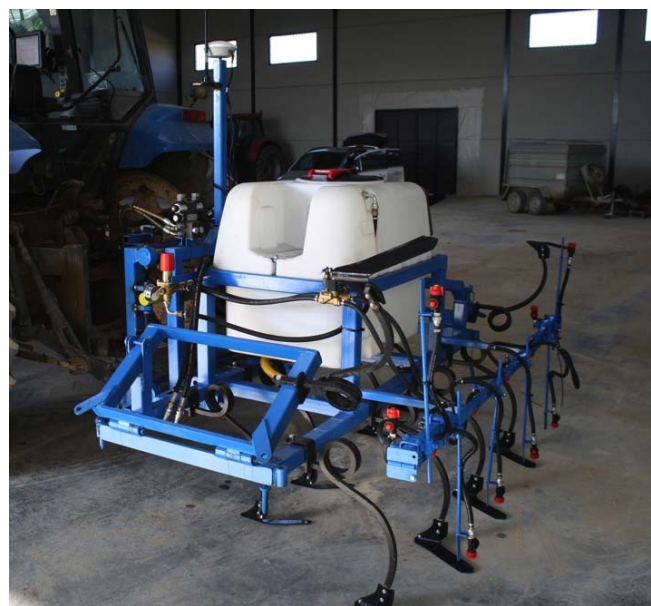
Figure 4. Prototype of six-row mechanical weed control cultivator for inter-row areas and band spraying for intra-row areas.
