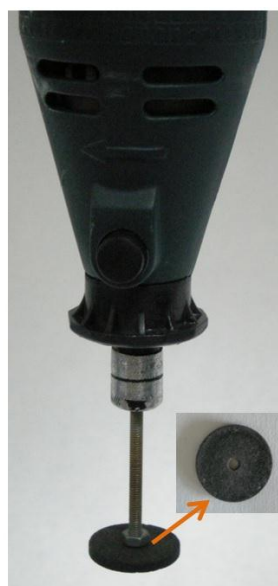
Figure 11. Borosilicate disk modified with carbon nanohorns extraction device. Reproduced with permission of from [67], copyright Elsevier, 2014.
