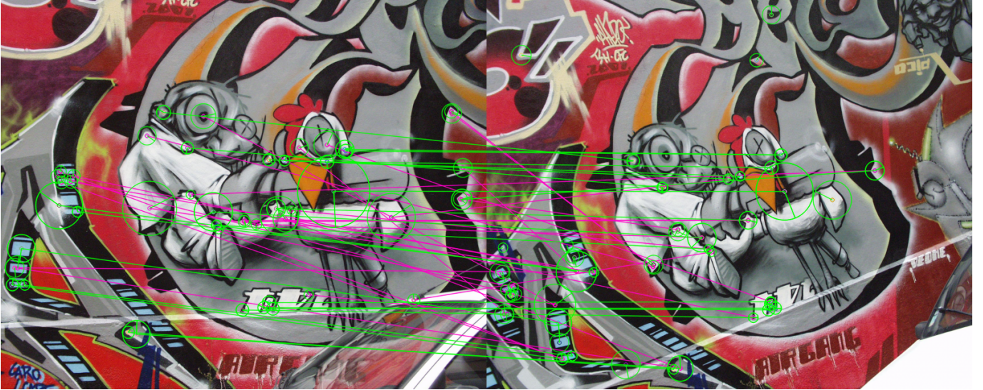
Figure 1: Keypoint matching example from the Oxford dataset [2]. Two images of the same scene taken from different angles. Keypoints in both images are represented as circles. Green lines represent correct matches while pink lines are erroneous matches. (Best viewed in color)
