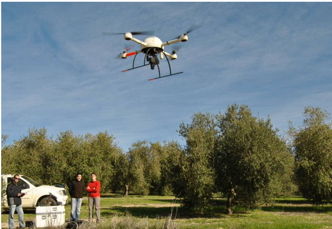
Figure 3. The quadcopter UAV and the visible-light (RGB) camera used to acquire the remote images of the olive plantation.
