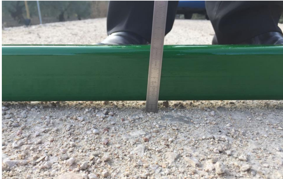
Figure 5.4: Rut depth measurement manually with straight edge and steel rule.
