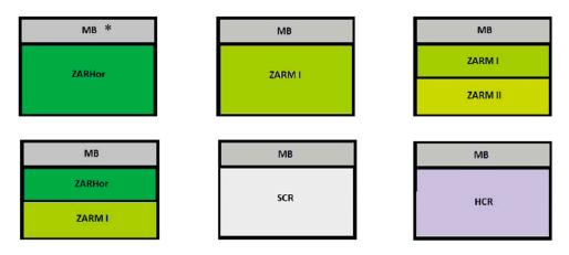
Figure 1. Types of structural sections recommended in the catalogue. \* MB = Bituminous mixture.
