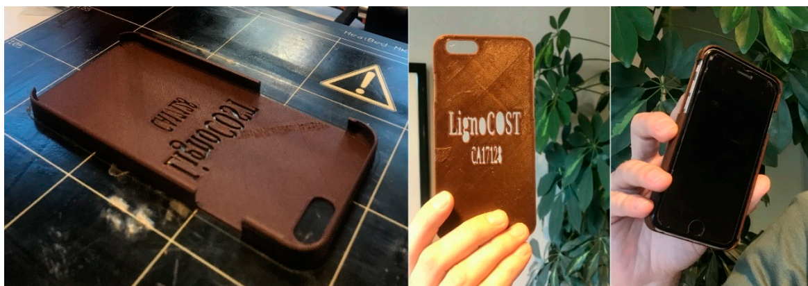
Figure 9. 3D printing of a smartphone protective case with PLA/lignin biocomposite filament.
