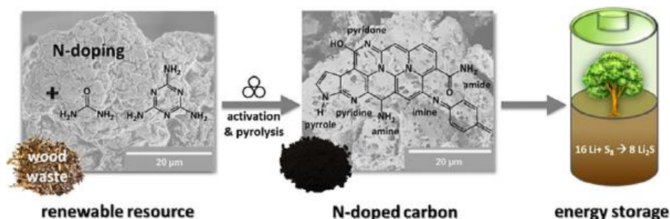
Fig. 10 Mechanical step and carbonization of a mixture of sawdust, urea and/or melamine and K_2CO_3 to prepare N-doped carbons as electrode for lithium-sulfur batteries. Reprinted with permission from Ref. [37] Copyright (2019) Wiley-VCH.
