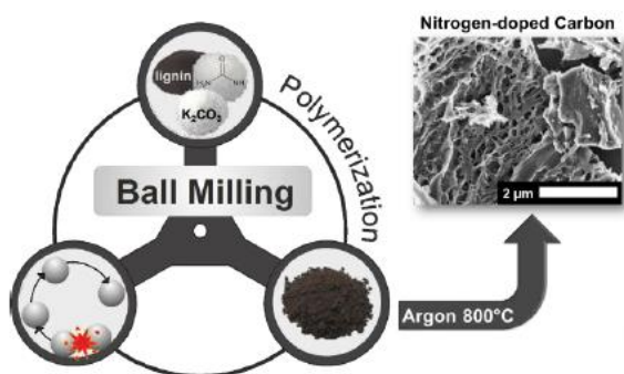
Fig. 9 Pictorial representation of the synthetic procedure of N-doped porous carbon. Reprinted with permission from Ref. [36] Copyright (2017) Wiley-VCH.
