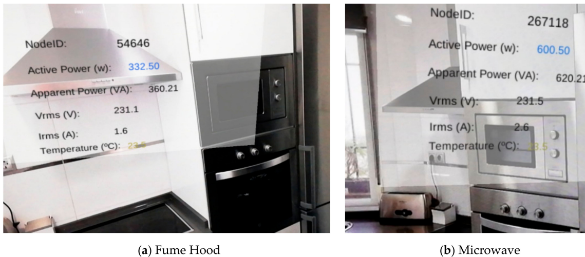
Figure 9. Augmented energy information displayed on the screen of the smartphone.
