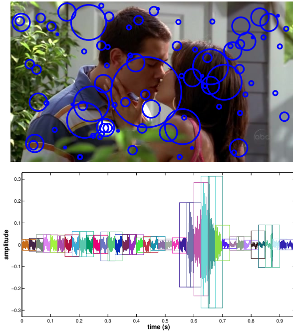
Fig. 5: Local audio-visual features. (top) Spatio-Temporal Interest Points (STIP) are used as basis for visual features. A HOG/HOF descriptor is computed for each STIP. (bottom) Audio signal is divided into overlapping frames . In this example, the signal is divided in frames of 0.05 seconds overlapping 0.025 s. Features are extracted over each audio frame. Then, each resulting feature vector is assigned to a word of the corresponding dictionary.
