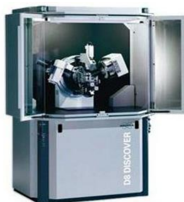
Figura 14. Equipo de DRX Bruker D8 DISCOVER, (imagen obtenida de “ https://www.bruker.com/products/x-ray-diffraction-and-elemental-analysis/x-ray-diffraction/d8-discover-family.html ”)
