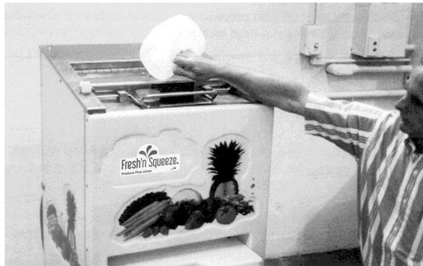
Water being poured into hole in hopper
