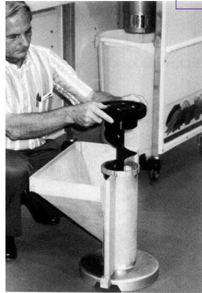
Figure 1d. Lifting screw out of hopper
