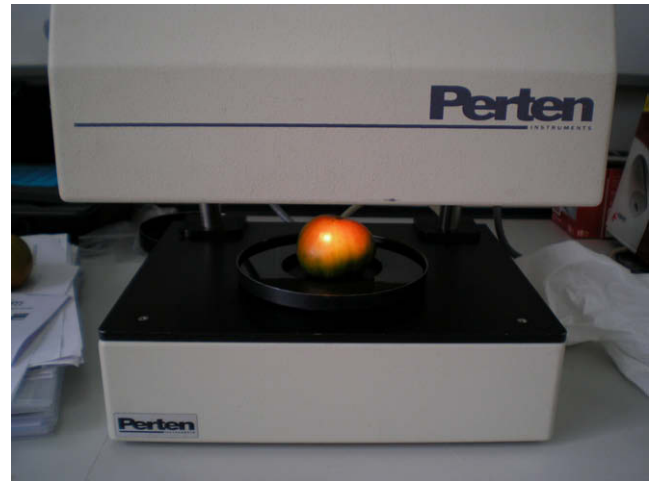
Fig. 3. Set-up of diode-array NIR spectrometer.
