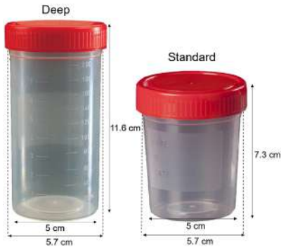
Figure 2 Deep and standard pitfall trap as used in the experiment.
