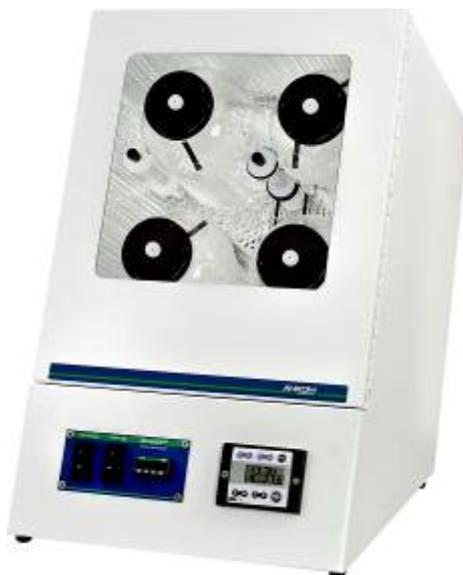
Figura 12. Imagen de Digestor/incubador Daysy (ANKOM Technology).
