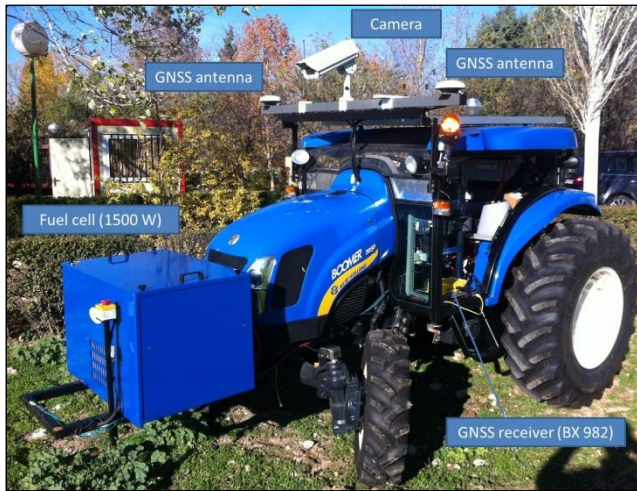
Figure 5.1. Autonomous tractor unit configuration.
