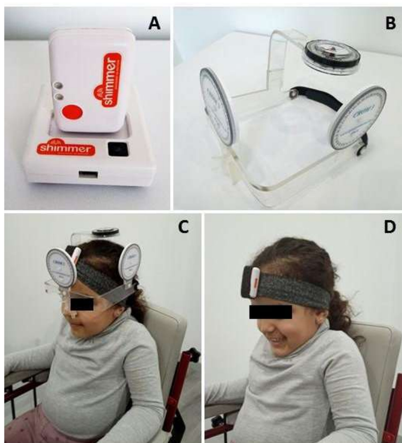
Figure 1. Devices and procedure of assessment. (A) Inertial Measurement Unit (IMU) Shimmer3 ® (Dublin, Ireland); (B) Cervical Range of Motion (CROM) 3 ® device (Lindstrom, Minnesota, USA); (C) positioning of IMU and CROM to assess craniocervical range of motion (first assessment on the first day); (D) positioning of IMU to assess craniocervical range of motion (second assessment on the first day, and assessment on the second day).
