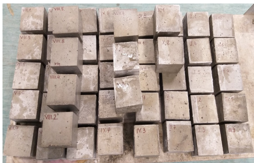
Figure 4. Concrete cubes prepared for testing.
