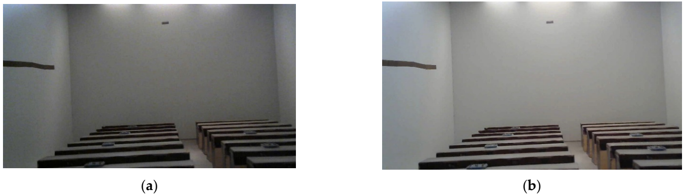
Figure 16. Qualitative comparative analysis of daylighting levels: (a) inside the scale model without heliostat illuminators; (b) the one with heliostat illuminators.
