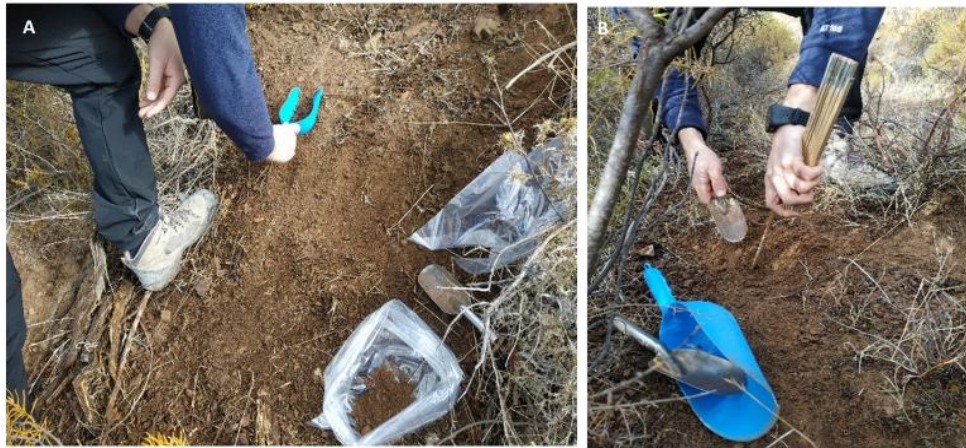
Figure 7 On the left, image A shows the shallow soil sampling (0 – 2 cm). On the right, image B shows the deepest oil sampling (2–5 cm).
