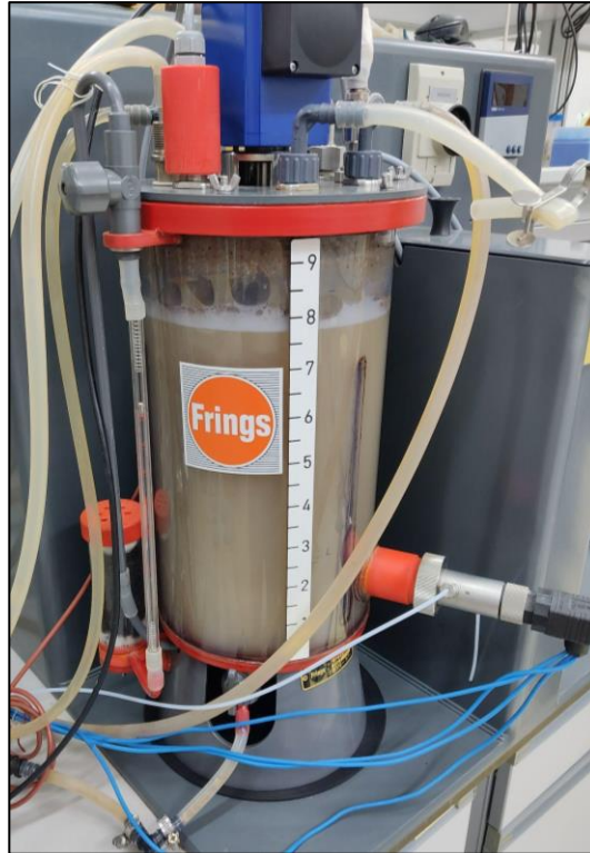
Figure 3. Bioreactor Frings on a pilot scale (effective capacity, 8 L) making wine vinegar. Source: own work.
