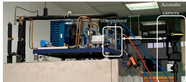
Figure 4. Noise measurement set up.
