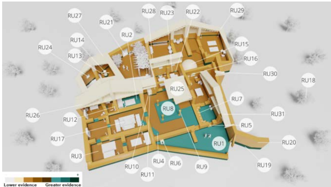
Fig. IV-4. Application of the evidence scale proposed by Ortiz et al. in the Baker's House virtual reconstruction.
