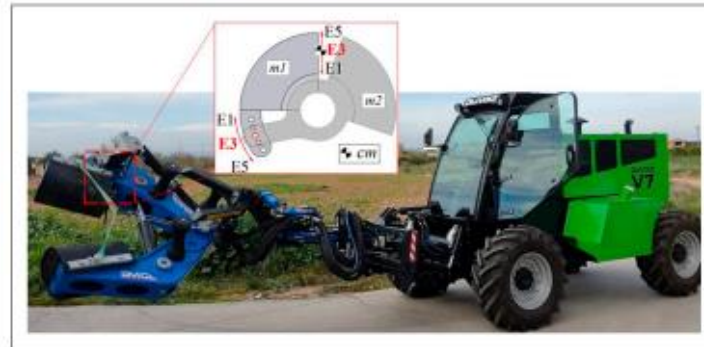
Figure 1. Trunk shaker developed by Talleres Mata Campos with configurable eccentricity to modify the vibration system's centre of mass (cm).
