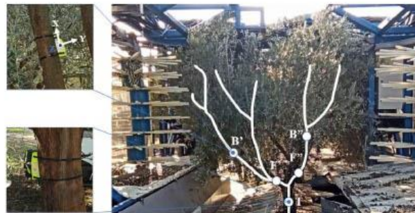
Fig. 3 – Accelerometers set in olives trees on the trunk (T), at the fork (F, F') and in branches (B, B').
