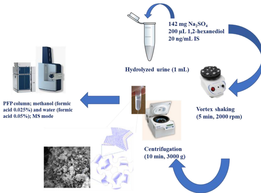
Fig. 1. Schematic of the SUPRAS-based sample treatment for screening analysis of multiclass substances in urine by LC-ESI-TOF.
