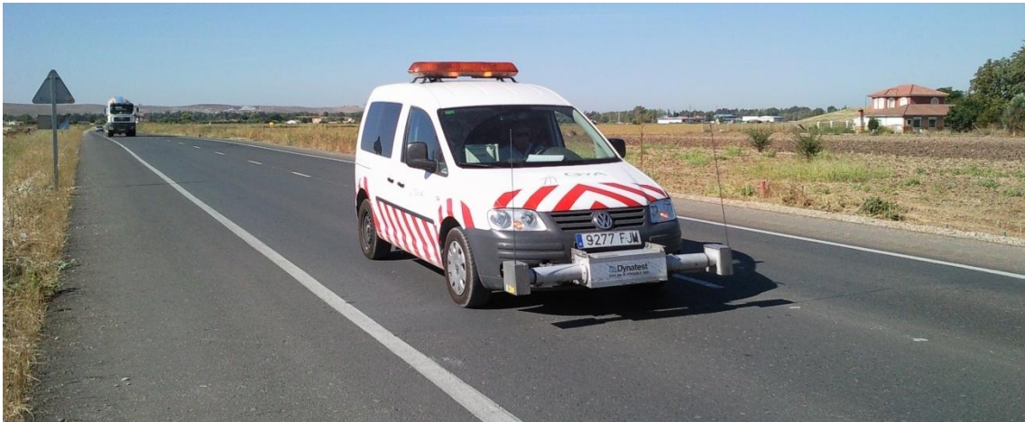
b). RSP MARK-IV equipment – Testing Roughness on ER on 2017
