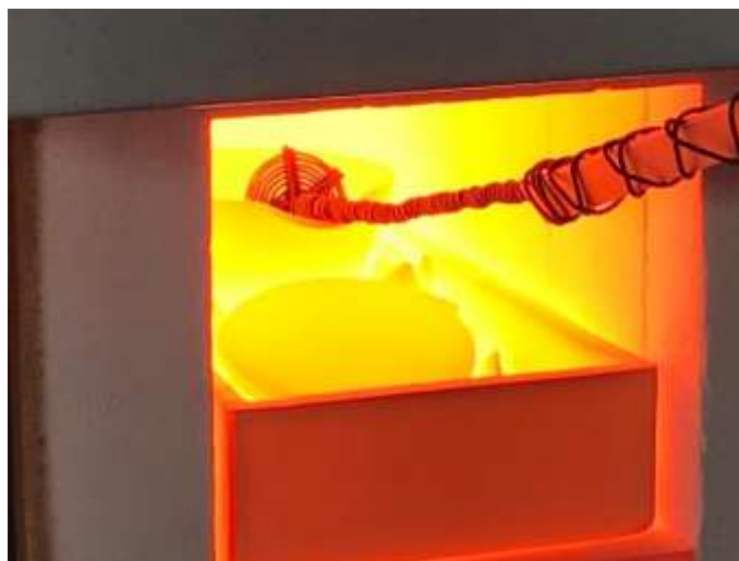
Fig. 3. EXP1 (step 6 of the recipe). Scum removal from the glass melt using an iron tool.
