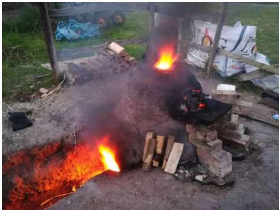
Fig. 1. Experimental Anglo-Saxon furnace in use. The furnace is shown here immediately after charging with fuel through the stoking hole (bottom left), the glass crucible containing the melt stood on a siege or shelf above and to one side of the fire chamber and could be accessed through the 'glory-hole' (centre-right) covered with a clay door.
