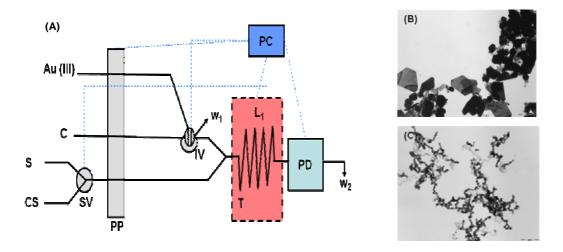
Figures B and C depict the TEM images obtained for the mixture of  $HAuCl_4$  and TGA in the absence and in the presence of TX-100 respectively. Figure B shows the formation of irregular polyhedral metallic clusters with a wide range of sizes, estimated between 60 and 300 nm. However the TEM image obtained in the presence of TGA and TX-100 shows the formation of spherical AuNPs with sizes in the range 10-40 nm.
