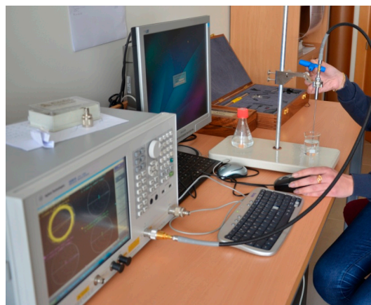
Figure 6. Keysight 85070E dielectric probe used for measurement of dielectric properties.
