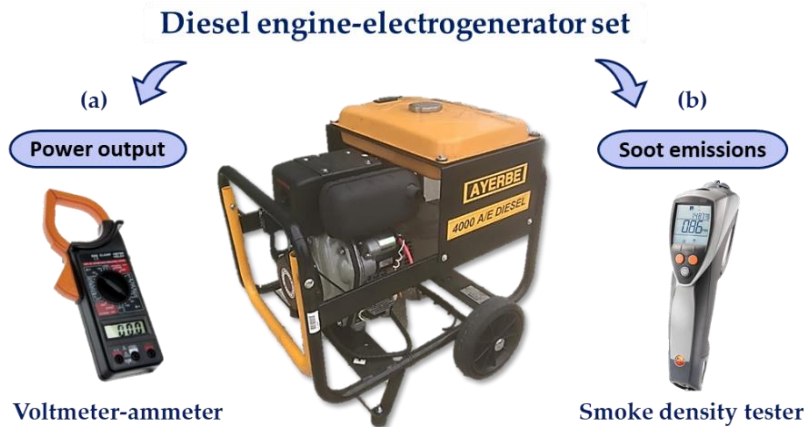
Figure 1. Scheme of experimental methodology to determine (a) power output by means of a voltmeter–ammeter device; (b) generated soot emissions by means of a smoke density tester, on a Diesel Engine-Electrogenerator Set [21].
