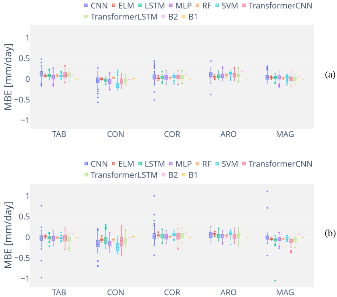
Figure 6.12. Boxplot with MBE values from all models and configurations in the different AWS, using 15 lag days (a) and 30 lag days (b)
