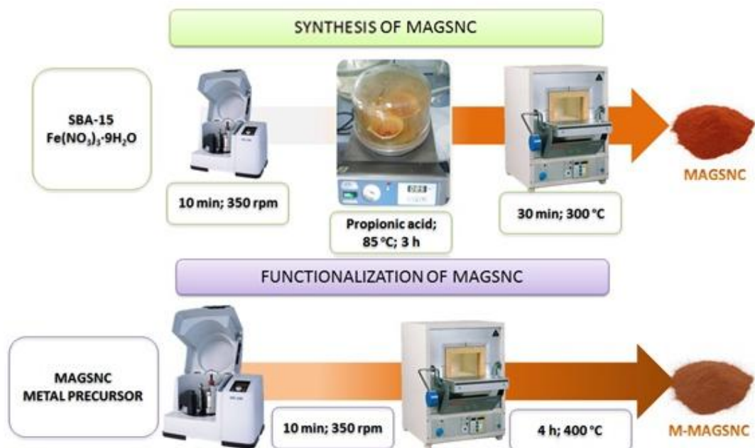
Scheme 1 Overview of the preparation of magnetic nanocomposites and further functionalization with metals.
