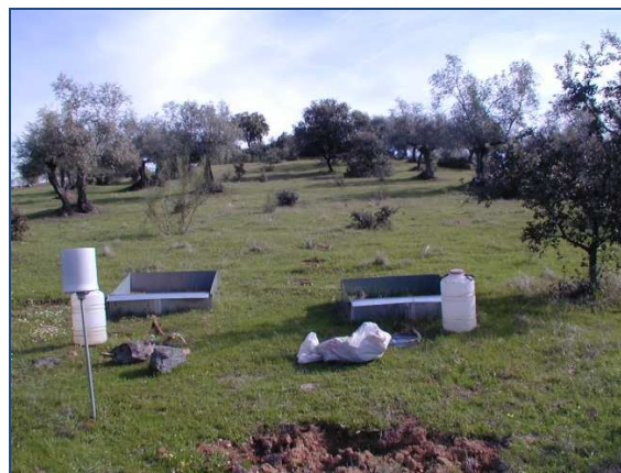
Fig. 2.2. Picture of a microplot block with conventional tillage, CT, and cover crop, CC, soil management, located at the Obejo farm, C5.
