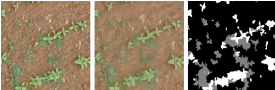
Fig. 4. Representation of the different steps for the procedure considered: image acquisition, segmentation of the image, and, finally, classification.
