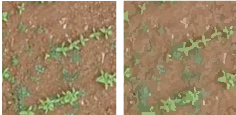
Fig. 1. The image on the left shows a region selected from the experimental field. The image on the right shows the output of the segmentation algorithm (note that objects have been plotted as regions with the same spectral information by measuring their spectral values).
